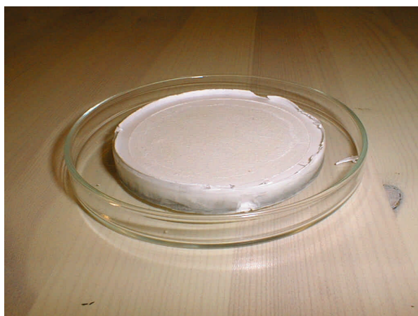
Figure 3.17. First successfully pressed sample of fluorohectorite. Picture taken by Magnus W. Haakestad.
