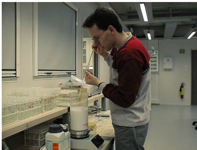
Figure 3.4. Clear water phase is sucked out.
