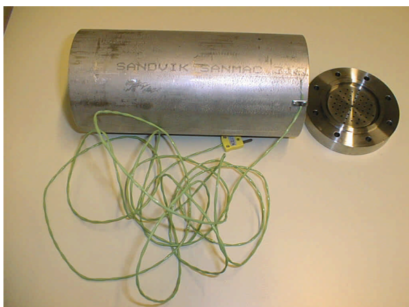
Figure 3.1. Outer cylinder with temperature element mounted
