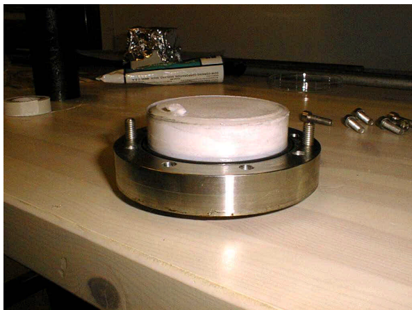
Figure 3.15. Pressed montmorillonite, still wet.
