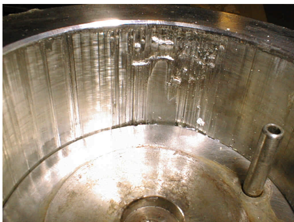
Figure 3.13. The inner cylinder is stuck.
