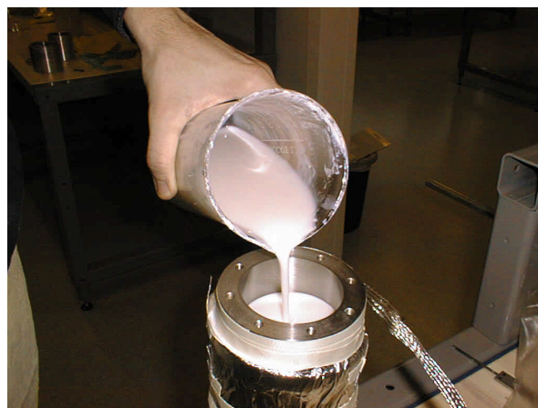
Figure 3.14. Montmorillonite is poured in.
