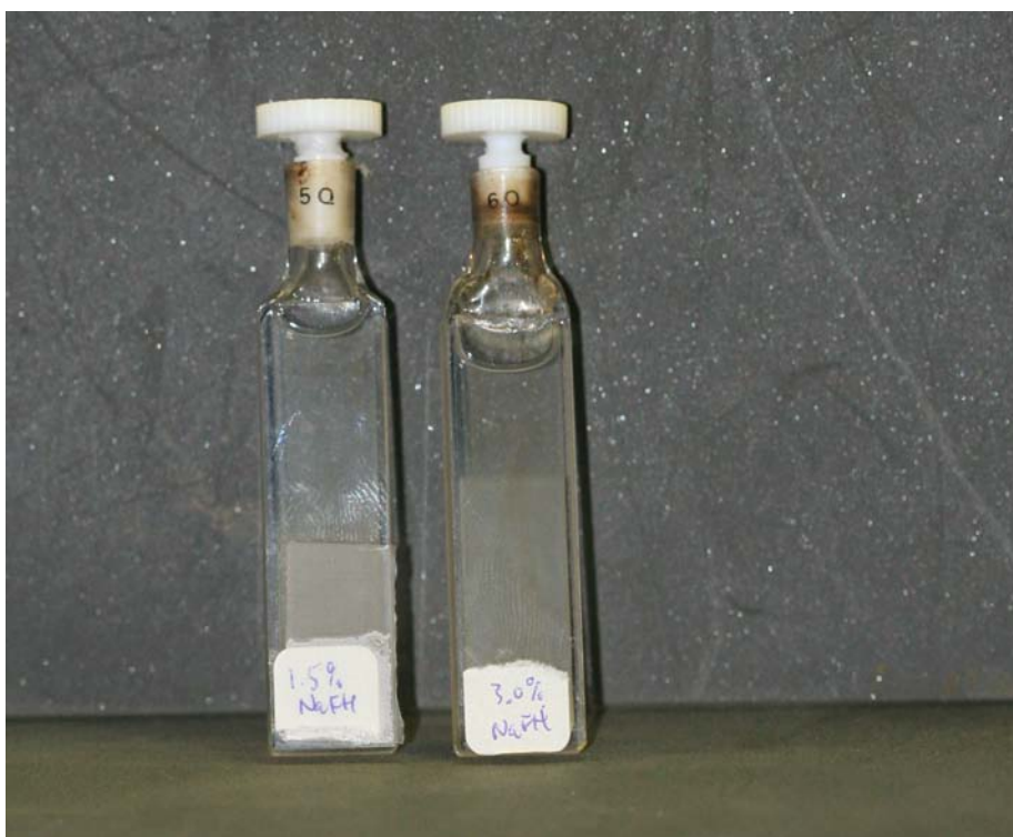
Figure 3.23: The new NaFH -solutions after four months of relaxation. One sees clearly that the lower concentrated phase is higher in the 3.0wt% (cuvette to the right) sample than in the 1.5wt% suspension (cuvette to the left).
