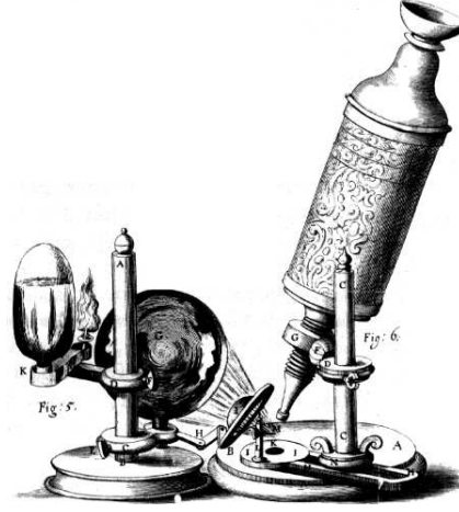
Figure 11: A sketch of one of Hooke's microscopes from 1665, lit up by a candle [31].
