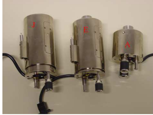
Figure 23: The three scanners for the MultiMode AFM, J, E and A.
