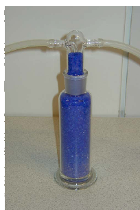
Figure 2.2: The silica gel dissicant, located before the TGA, supplies a dry atmosphere.
