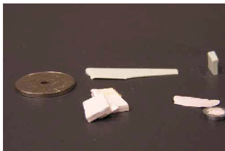
Figure 2.1: thin and thick samples of Fluorohectorites with a 1 Krone coin which provides the scale
