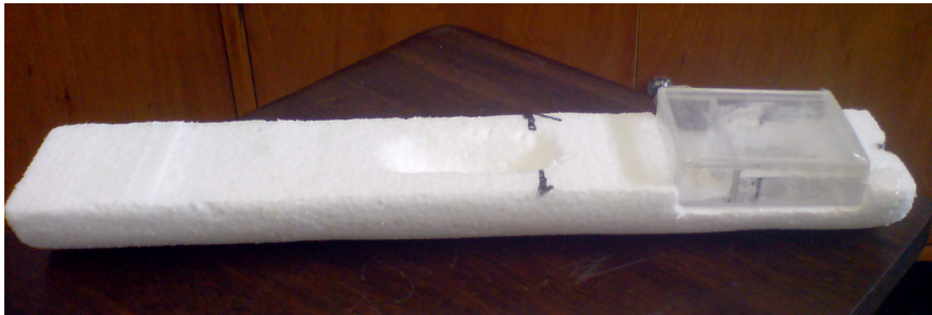
FIGURE 2.6: Image of the sample holder placed on the styrofoam half-cylinder used for insertion into the MRI system. Sample holder visible on the right.
