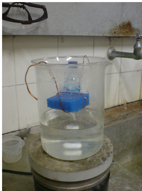
FIGURE 2.9: The resolution test sample placed over a beaker of boiling water.
