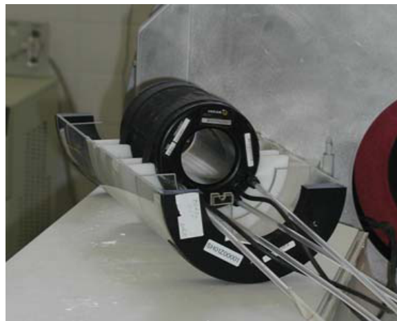
FIGURE 2.2: The Varian RF coil. When installed in the machine, the cylindrical axis of the saddle-type coil is along the axial bore of the magnet, i.e. the z -direction of the system. Taken from [65].
