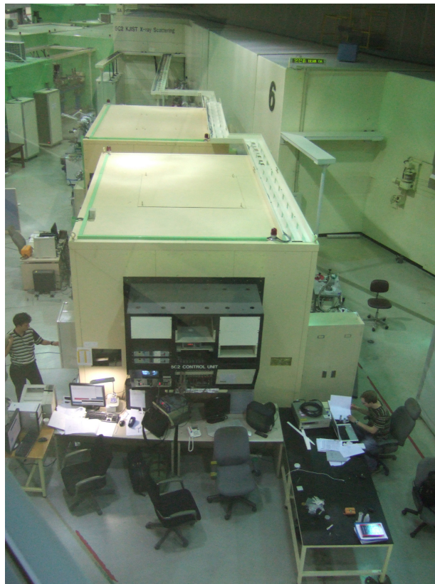
Figure 3.12: The KJIST X-ray Scattering beamline at Pohang Light Source, Pohang, South-Korea. Featuring two different beam outlets, 5C1 being the hindmost box seen here.
