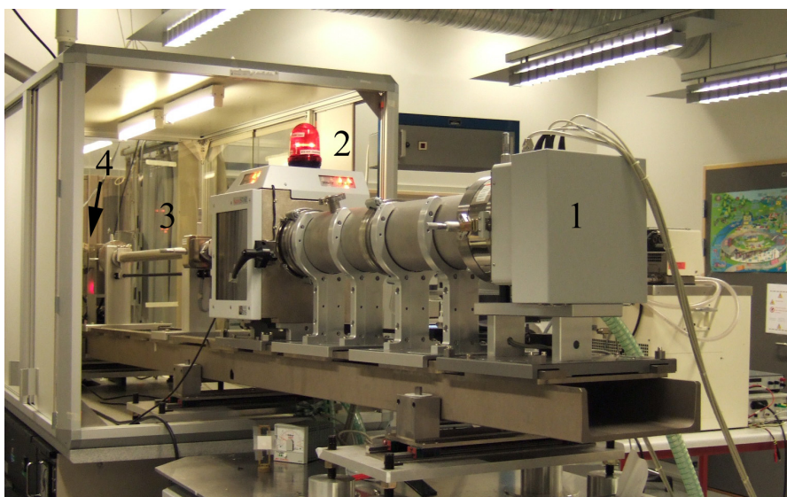
Figure 3.10: Components of the NanoSTAR system, 1. Rotating anode source, 2. Pinhole collimating system, 3. Sample chamber, 4. Detector.
