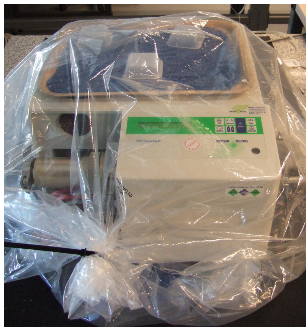
Figure 3.4: Setup of the TGA during measurements below room temperature, placed inside a plastic bag with supplies of silica gel.
