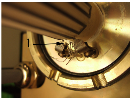
(a) Base: 1. Temperature sensor, at the end of a coil of wires.
