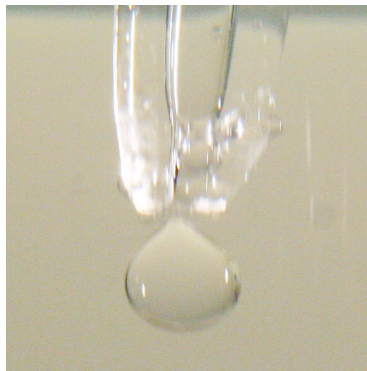
Figure 9: Pendant drop hanging from a burette with tip diameter of 4mm. 100 cSt silicone oil drop in sunflower oil (!).
