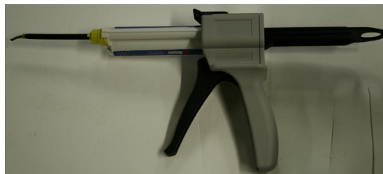
Figure 3.7: Dispensing gun for dispensing RepliSet silicon rubber casting compound. A cartridge and mixing nozzle is mounted on the gun.
