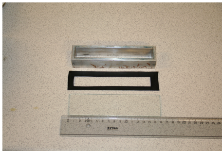
Figure 3.10: The three parts of a mould; glass plate, rubber seal, and aluminium frame.
