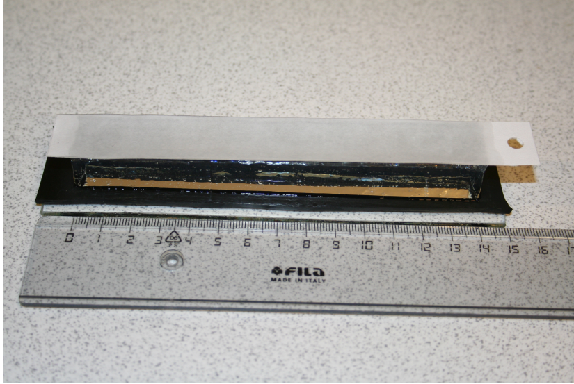
Figure 3.3: A gel sample with a strip of filter paper placed on the top surface. This picture was taken after approximately 5 minutes and the filter has absorbed water from the sample.
