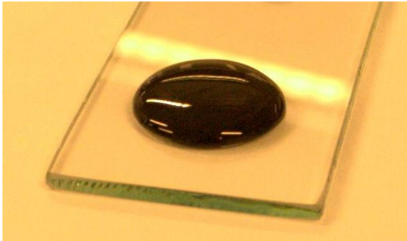
Figure 4.16: The casting compound applied on a glass plate to. It should be noted that the light from a lamp in the ceiling is reflected on the surface of the glass plate. The focus is however on the casting material and not on the reflected image of the lamp.
