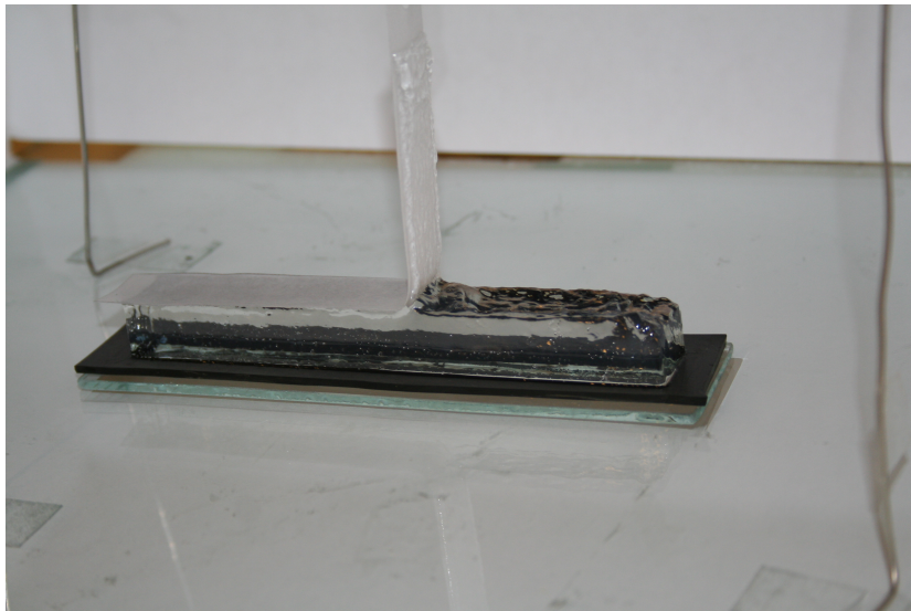
Figure 3.4: A gel sample undergoing fracture. The filter paper is pulled upwards and a thin layer of gel is peeled off the rest of the sample, causing a fracture to propagate horizontally through the sample.
