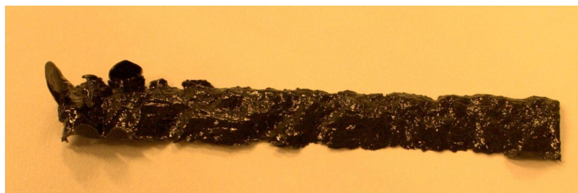
Figure 4.20: A replica similar to the replicas that were analysed with laser profilometry.
