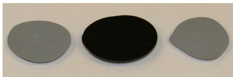
Figure 4.19: Three different replicas of rough surfaces. The middle replica is made using RepliSet F1 compound, while the two others are made using the grey RepliSet GF1 compound.
