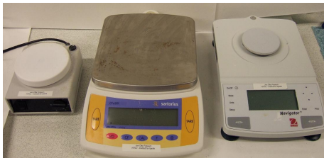
Figure 3.11: From the left: The Heidolph MR1000 magnetic stirrer and the Ohaus Navigator N30330 and Sartorius CP 6201 electronic balances.
