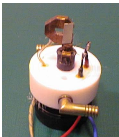
Figure 3.8: Sampleholder for x-ray diffraction measurements on fluorhectorite under a controlled atmosphere
