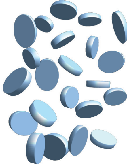
Figure 2.8: The microscopic order of the isotropic phase of a disc-like nematogen. There is no orientational or positional order.
