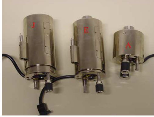
Figure 18: The three scanners for the MultiMode AFM, J, E and A.
