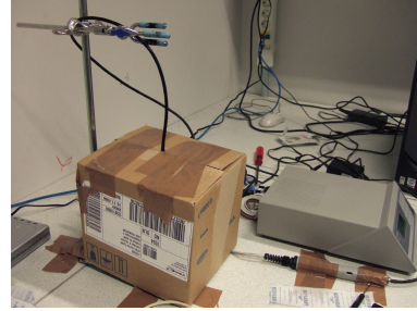
(b) Setup covered with a cardboard box, the hygrometer with probe handle is shown in the lower right corner.
