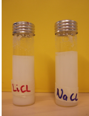
Figure 4.3: Salt slushes used for calibration of hygrometer probe.
