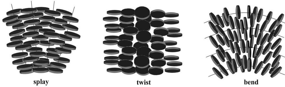
Figure 1.7: The three basic types of deformation of the director field: splay, twist and bend. The shapes represent disk-like particles that are viewed edge on with the face normal as the director. In all three cases, deformation is present in the plane of the page. There is no change in the director orientation in going into or out of the page. When disks are fully viewed edge on, they may look like rods oriented perpendicular to the director. For this representation the formation of the bend and splay distortion interchange.
