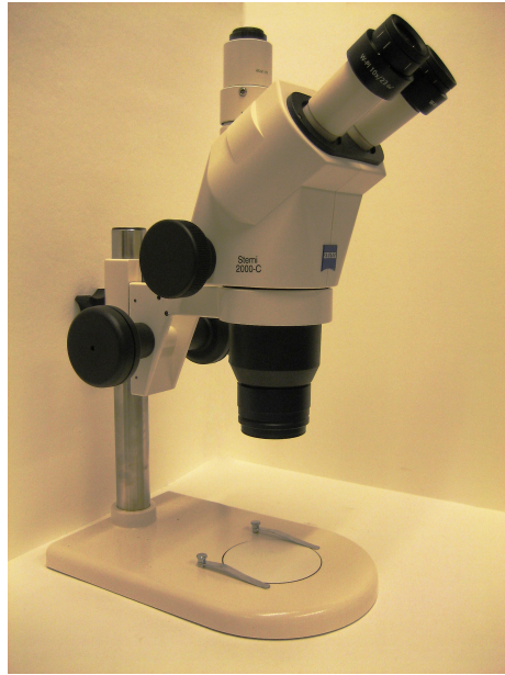
Figure 4.5: Zeiss Stemi 2000C microscope with an additional 2x magnification lens attached to it.
