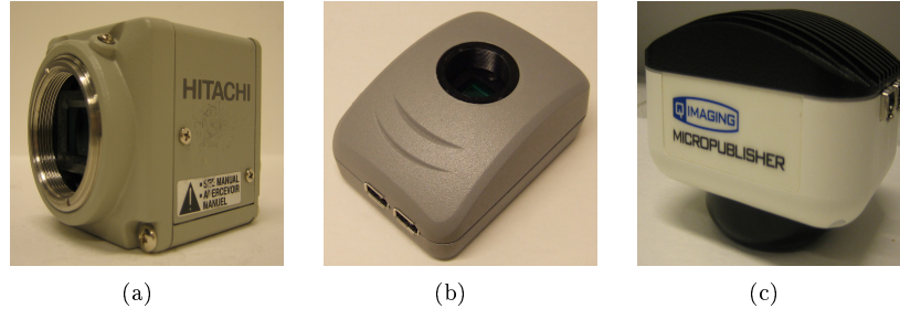
Figure 4.4: Three different digital cameras used together with the Zeiss optical microscope: (a) The Hitachi camera, (b) the PixelLink camera and (c) the Q-imaging camera.
