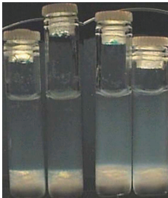
Fig. 4. Example of Na-fluorohectorite samples (3 w/w% clay) viewed when placed between crossed polarizers. The two leftmost samples: 2 \times 10^{-3} M, the two rightmost samples 6 \times 10^{-3} M.
